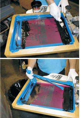
While screen is clamped into press, scrape out leftover ink with an "INK KNIFE" and return it to the ink bucket.
