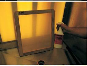
Spray both sides of screen liberally with "BOB'S HAZE REDUCER AND DEGREASER". Scrub in a circular motion with a "SCREEN BRUSH". (Do not use the same brush used for reclaiming. This will prevent screen contamination.) Rinse screen brush thoroughly between screens to prevent contaminants from one screen being carried to the next.
