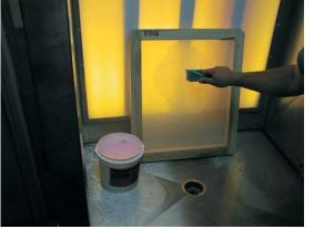
Wet screen mesh with cold water. Apply "BOB'S MESH ABRADER" to screen mesh. Use a clean "SCREEN BRUSH" and scrub in a circular motion. Repeat on second side. (This step removes oils and contaminants from the new screen mesh and allows the emulsion to adhere better to the mesh. This process can be repeated as often as needed, whenever emulsion is experiencing difficulties adhering to mesh.) Abrading after every 10 to 20 reclaimings is recommended.
